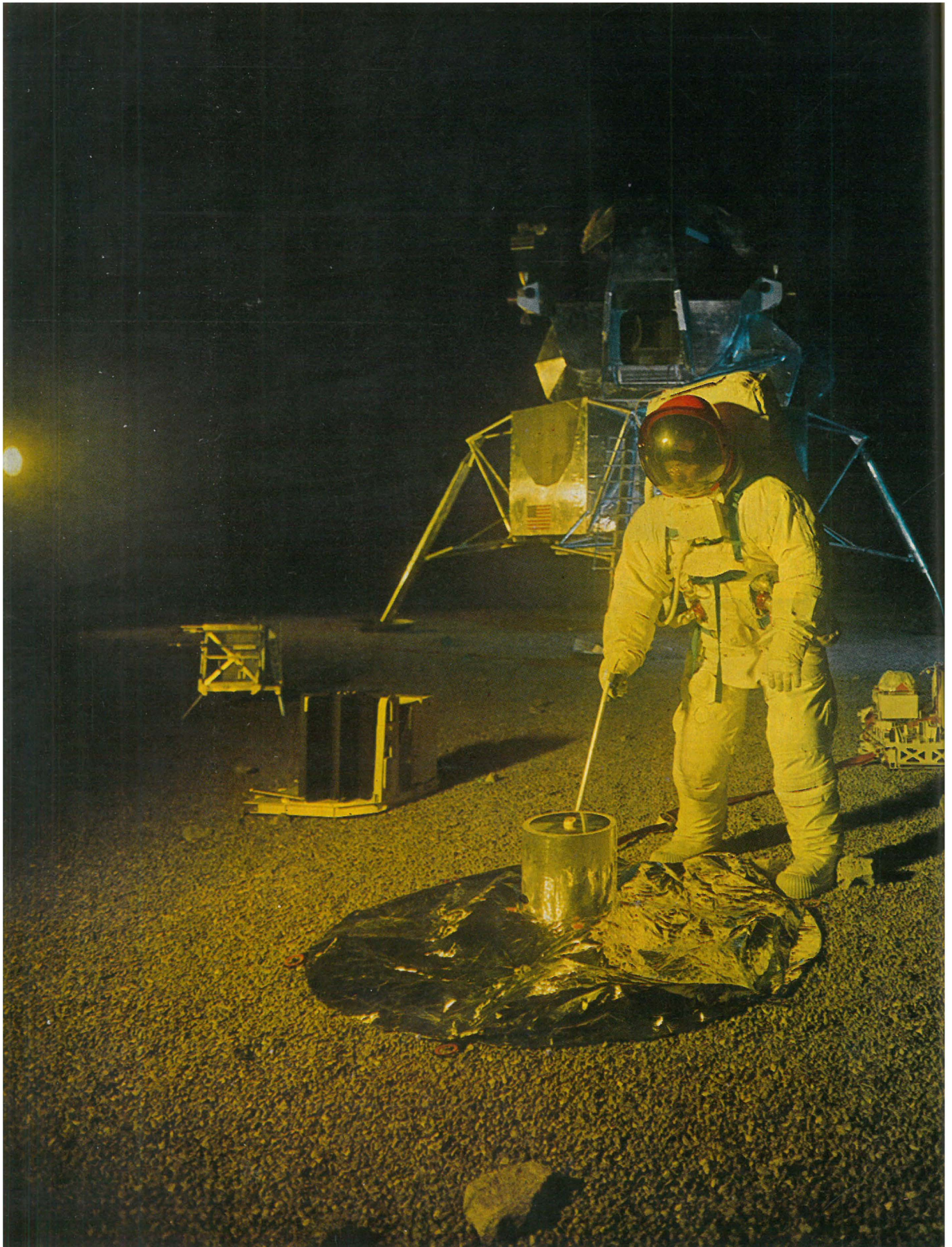
In eerie light of a lunar sunrise, Astronaut Don Ling works outside a Lunar Module set on a realistic lunar landscape. He is setting up an instrument to measure moonquakes, using a hook-ended rod because of the difficulty of bending and kneeling
