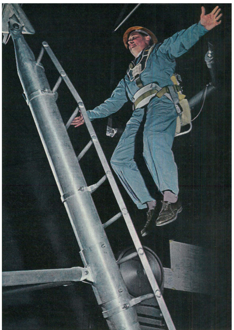
Practicing the semi-weightlessness of moon walking, Engineer Harold Johnson romps on NASA's "Partial Gravity" simulator, which he helped invent to duplicate the effect of moon's gravity.
